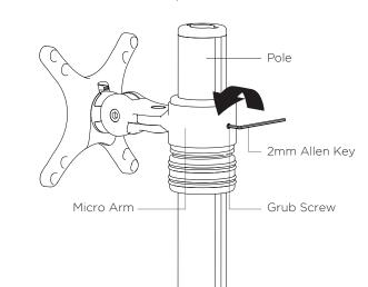
Step 2: Re-insert the Grub Screw previously removed. Turn the Grub Screw clockwise until it is tight. Do not over-tighten Slot in Pole Grub Screw Hole (0)2mm Allen Key Grub Screw
