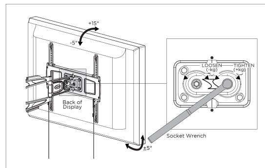
Position your display to the desired viewing angle using the angular movement allowed by the double ball mount.
