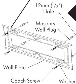
**TIP: Use a spirit level to ensure the wall plate is horizontal**
