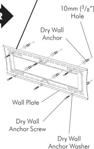
**TIP: Use a spirit level to ensure the wall plate is horizontal**
