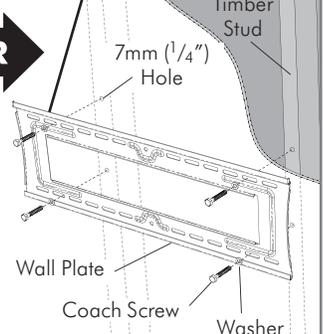
**TIP: Use a spirit level to ensure the wall plate is horizontal**
