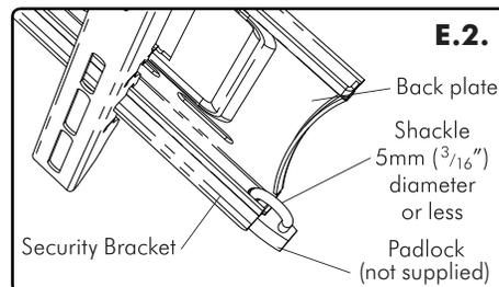
For additional security, it is suggested that a Padlock is attached through the Security Bracket and the Wall Plate on either side as shown. The Padlock (not supplied) should have a shackle diameter no larger than 5mm ( $\frac{3}{16}$ ").
